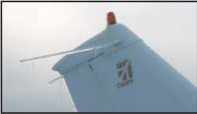
Ice can cause antennas to vibrate so severely that they break
