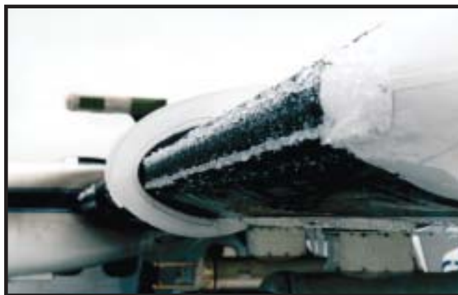
Clear ice formation on wing leading edge
