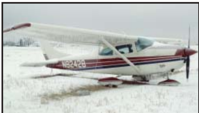
Remove all frost, snow, or ice from the wings
