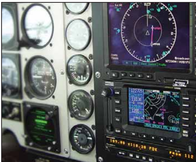
Multifunction displays can do a lot more than just display GPS data. This one, for example, is showing traffic information derived from ADS-B.
