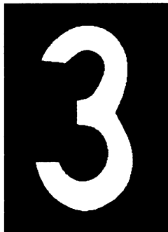
Figure 22. Typical Runway Distance Remaining Sign
