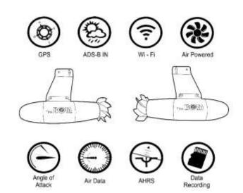
Once it is installed, the BOM connect via Wi-Fi to a tablet inside the cockpit and data can be displayed on multiple Apps thanks to its open protocol.
