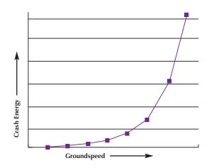
Energy increases with the square of speed. A 60-knot landing is only 50 percent faster than a 40-knot landing, but involves 125 percent more energy.
