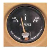
If your aircraft doesn't have warning lights for charging system malfunctions, include the ammeter in your regular instrument scan. Consider adding a warning light as your next upgrade.
