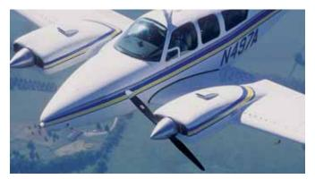
Feather the "dead" propeller in a twin after verifying that the engine has indeed failed. At low altitudes or airspeeds, it may be necessary to feather immediately.
