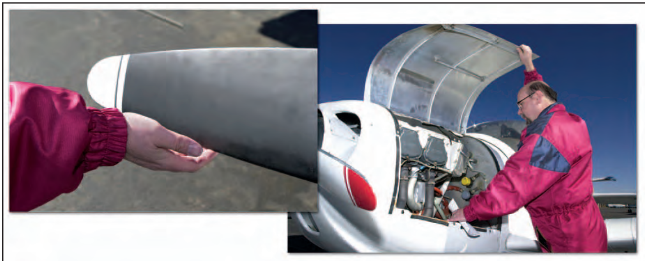
Figure 2-8. Check the propeller and inside the cowling.
