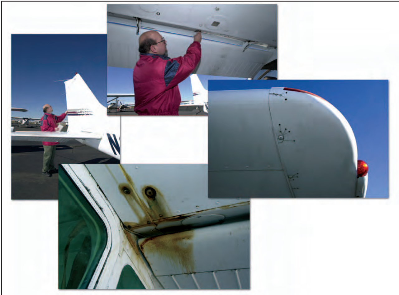
Figure 2-6. Wing and tail section inspection.
