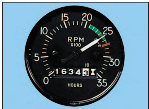
Figure 5-5. Engine r.p.m. is indicated on the tachometer.
