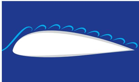
SMOOTH BOUNDARY LAYER AIRFLOW OVER AIRFOILS IS CRITICAL TO SAFE FLIGHT—DEGRADE IT WITH ANY SNOW, FROST, OR ICE AND FLIGHT MAY NOT HAPPEN.
